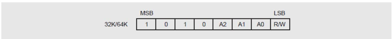
Figure 4: Device Address
