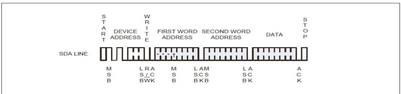
Figure 5: Byte write
